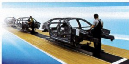
The Skid Transfer System
